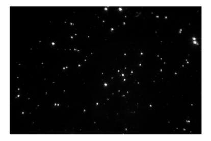
Each image point in the central region of the image field should be perfectly circular and comprise a circular disc with one or two faint rings around the outside. This is the diffraction limited Airy disc. You will be confident that you have correctly aligned the objective when this condition is reached and when the rings remain continuous and circular each side of best focus.
