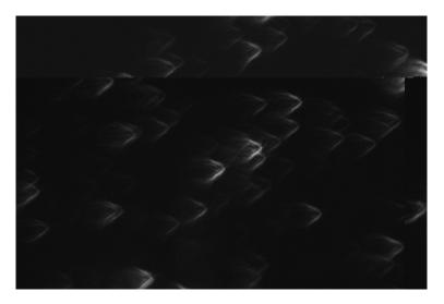
The point images are comet-like because misalignment causes coma to be introduced. The differing brightness occurs because the pinhole sizes range from approximately 0.5 to 5 microns diameter.
